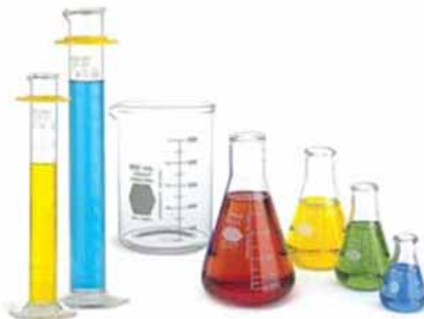
FIGURE 1.5 Graduated Cylinders, Beakers and Erlenmeyer Flasks:
