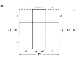
The dimensions, in inches, of the box are 12 - 2x by 12 - 2x by x. The volume is the product of the dimensions (volume = length × width × height):
