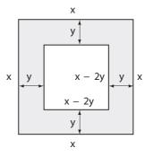
The area of the large square is  $x \cdot x$ , or  $x^2$ . The area of the small square is (x - 2y)(x - 2y), or  $(x - 2y)^2$ .
